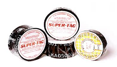
PVC tape specially designed for flame retardance and toughness. Made to adhere to portable cable jacket materials. Dielectric rating - 1000 Volts per mil. Meets or exceeds all U.L. requirements. Printed tape meets M.S.H.A. acceptance # P-07-KA050001-MSHA.
